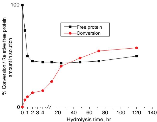
**Figure 14.2** A typical profile of cellulose hydrolysis progression and relative amounts of free protein in solution over hydrolysis time.
