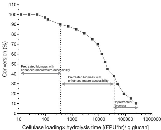
**Figure 14.6** Hypothetical depiction of cellulose conversion versus cellulase loading  $\times$  hydrolysis time (FPU hr/g glucan) with changes in macro-/micro-accessibility in pretreated biomass.
