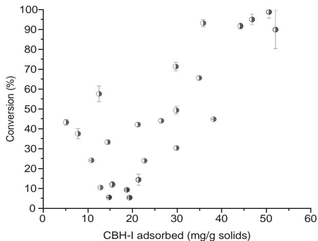
**Figure 14.5** The 24-h cellulose conversion (%) versus CBH-I adsorption (mg/g solids) for Avicel cellulose and poplar solids prepared by various leading pretreatments and those solids hydrolyzed to different extents (Data adapted from Kumar and Wyman [42]).
