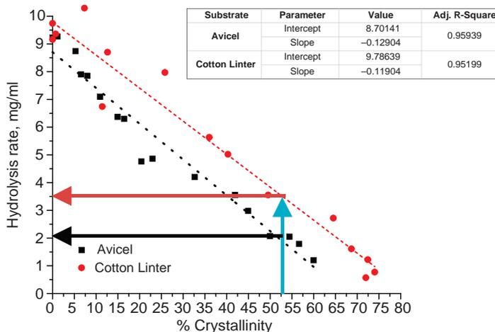
**Figure 14.4** Hydrolysis rate versus crystallinity for two cellulose substrates with different initial DPs. Cellulose samples of different crystallinities were prepared at varying phosphoric acid concentrations (Data re-plotted from Bansal *et al.* [236])
