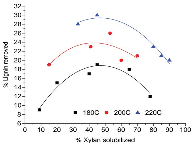
**Figure 14.3** Relationship between the amount of lignin removed (% of original) and xylan solubilized for batch hydrothermal pretreatment of corn stover performed at various temperatures and times (Data adapted from figure 14.6 in Liu and Wyman [165]).
