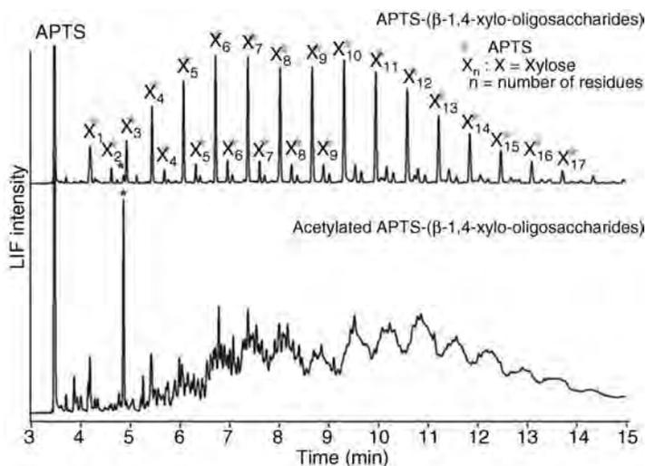
**Figure 19.8** LIF-electropherograms of APTS derivatized  $\beta$ -(1, 4)-xylooligosaccharides (top) and (less diluted) O-acetylated  $\beta$ -(1, 4)-xylooligosaccharides (bottom) obtained from hydrothermally treated *Eucalyptus* wood (\* is maltose internal standard). (From Kabel *et al.* [115] with permission from Elsevier).
