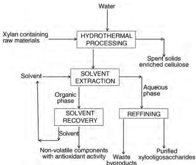
**Figure 19.2** Hydrothermal treatment coupled with solvent extraction for production of purified XOs from xylan-containing lignocellulosic materials. (Adapted from Moure et al. [45] © 2006, Elsevier).
