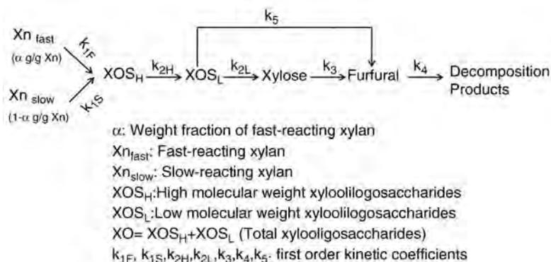
**Figure 19.1** Xylan reaction pathway in autohydrolysis to oligomers, xylose, furfural, and degradation products. (Adapted from Parajo et al. [28] © 2004, Elsevier).
