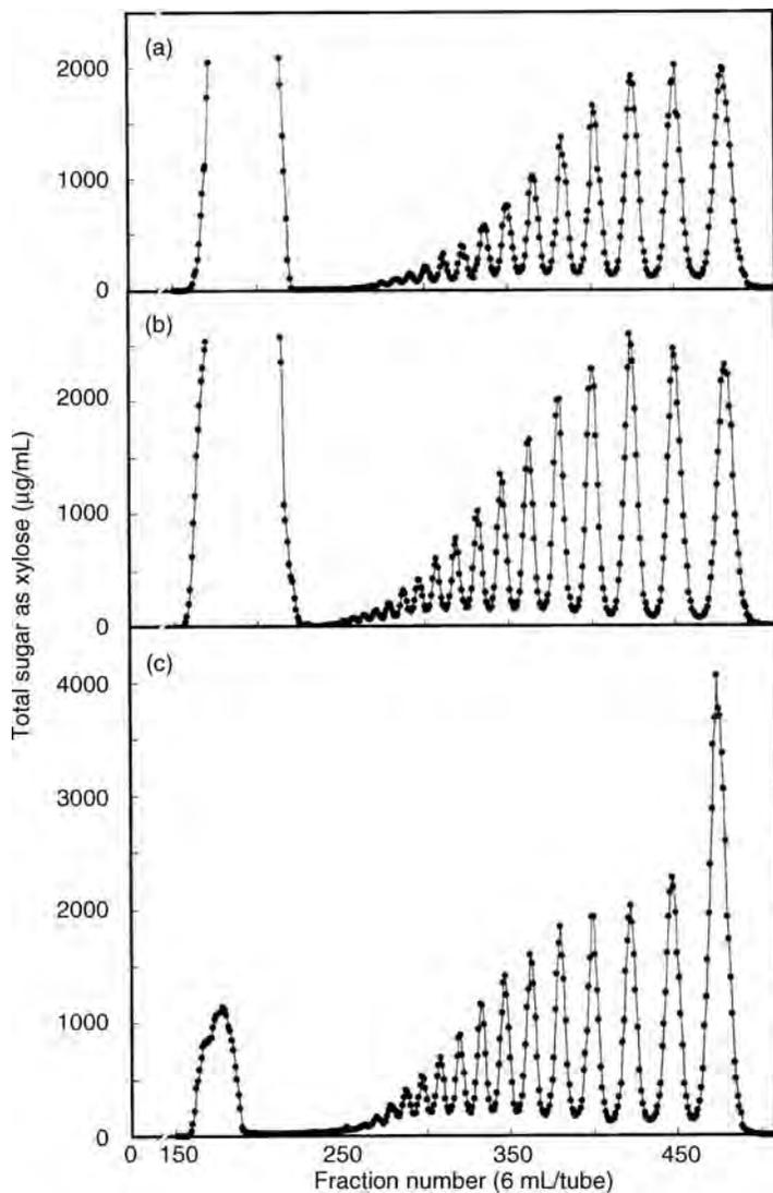
**Figure 19.3** Elution profiles of hydrolysis products of three kinds of xylans on BioGel P-4 and Toyopearl HW-40F columns connected in series: (a) cottonseed xylan; (b) birchwood xylan; and (c) oat spelt xylan. (Adapted from Sun et al. [42] © 2002, Elsevier).
