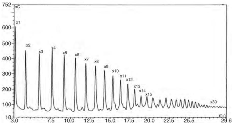
**Figure 19.7** Dionex IC chromatogram of xylooligosaccharides released from hydrothermal pretreatment of corn stover. (From Yang and Wyman [2] with permission of Elsevier).
