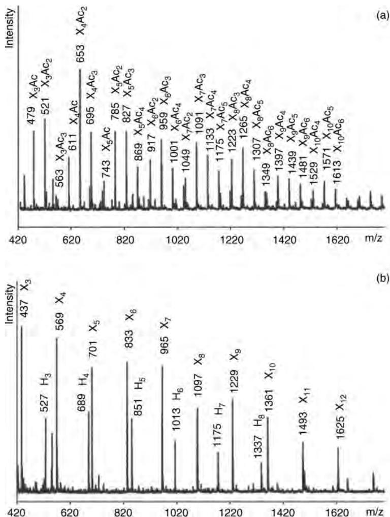
**Figure 19.9** MALDI-TOF mass spectra of the neutral xylooligosaccharides obtained from Eucalyptus wood hydrolysate (a) before and (b) after saponification ( $X$  = xylose;  $Ac$  = acetyl-group;  $H$  = hexose). (From Kabel et al. [123] with permission from Elsevier).
