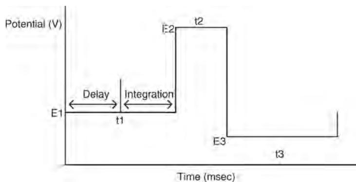
**Figure 19.6** Diagram of the pulse sequence for carbohydrate detection on a PAD detector. (Reproduced with permission of Dionex Corporation).
