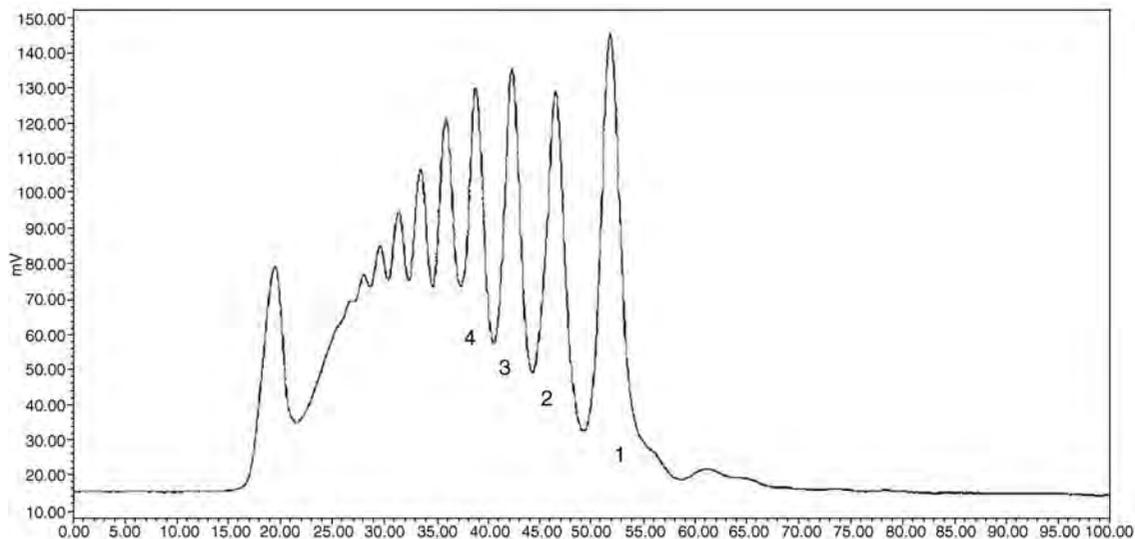
**Figure 19.4** IMP chromatogram of xylooligosaccharides derived from hydrothermal pretreatment of oat spelt xylan. 1: DP1; 2: DP2; 3: DP3; 4: DP4. (From Li et al. [89] with permission from Springer).
