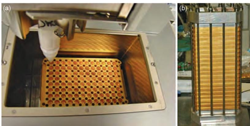
**Figure 22.4** The NREL HTPH reactor system uses the Symyx Powdernium to dispense biomass into (a) the wells of the 96-well reactor plate with a reaction mass of 255 mg per well with (b) 20 reactor plates stacked together in a modified 2-gal Parr reactor for pretreatment. (Reproduced from Decker et al. [12]).
