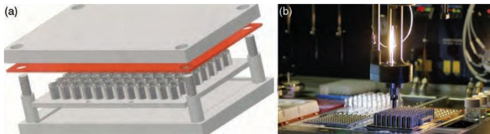
**Figure 22.3** UCR's HTPH reactor system [25] including the original reactor design in which Hastelloy wells with a 250 mg reaction mass were (a) press fit into an aluminum plate clamped between two stainless steel plates during pretreatment, and (b) the updated reactor with larger free-standing Hastelloy wells (450 mg reaction mass) being loaded by a Symyx Core Module.
