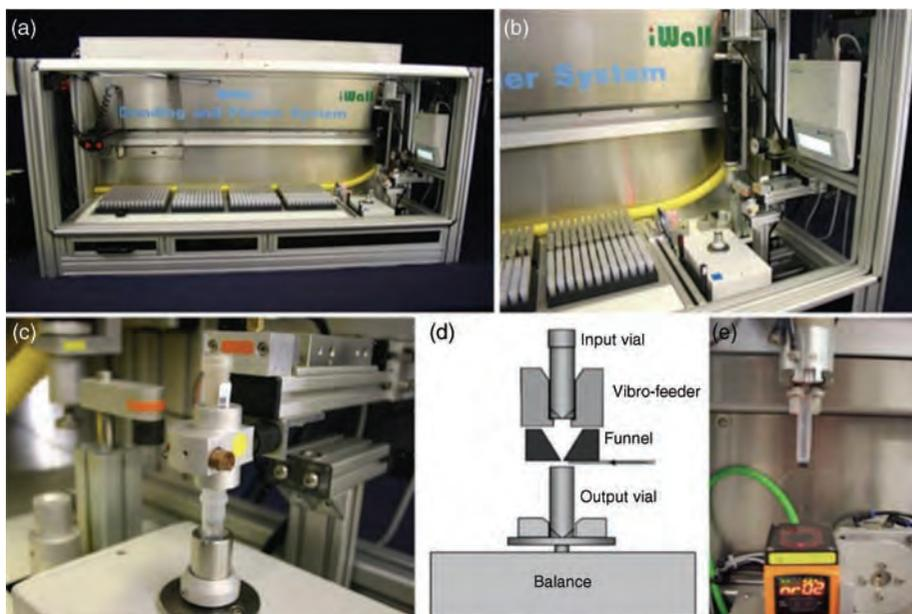
**Figure 22.5** GLBRC's HTPH system, including (a) iWall robotics platform for milling and dispensing. More detailed views of the (b) weighing substation, (c) balance and vibro-feeder dispensing from input (upper) to output (lower) tube, (d) diagram of weighing substation, and (e) bar code scanner substation are also shown. (Reproduced from Santoro et al. [23] with permission from Springer).
