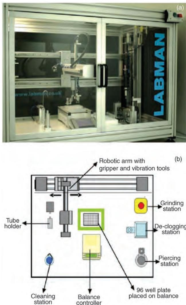
**Figure 22.6** HTPH system described by Gomez et al. including (a) general view of robotics platform for milling and dispensing and (b) schematic of robot's different substations. (Figure obtained from Gomez et al. 2010 [22]).
