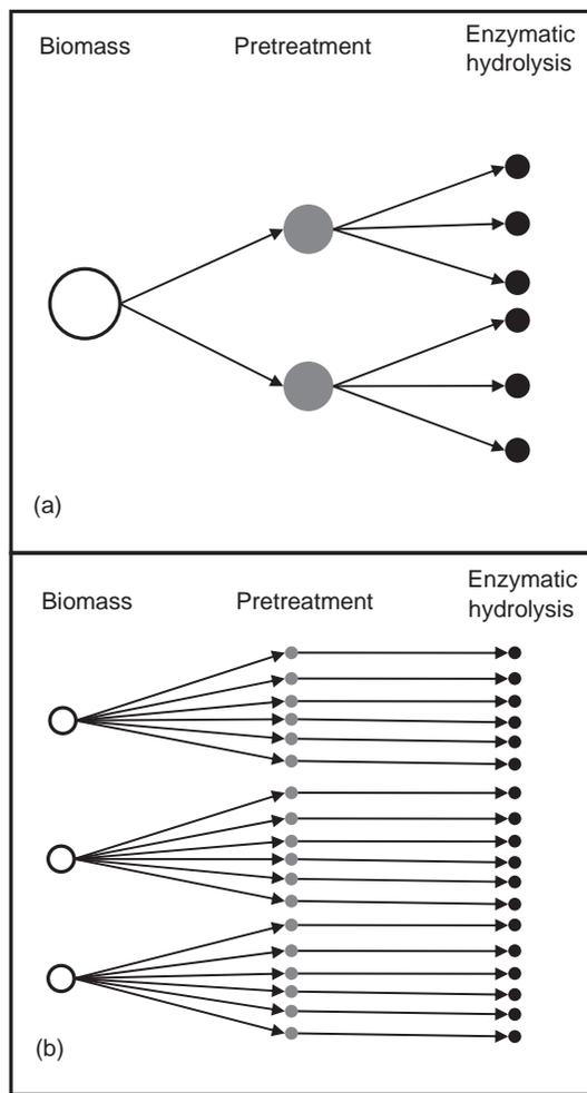
**Figure 22.1** Comparison of (a) conventional pretreatment and subsequent enzymatic hydrolysis laboratory experiments with (b) HTPH approach, in which the same reactor is employed for both pretreatment and enzymatic hydrolysis to avoid processing between the two operations. (Adapted from Studer *et al.* [26] © BioMed Central Ltd.).
