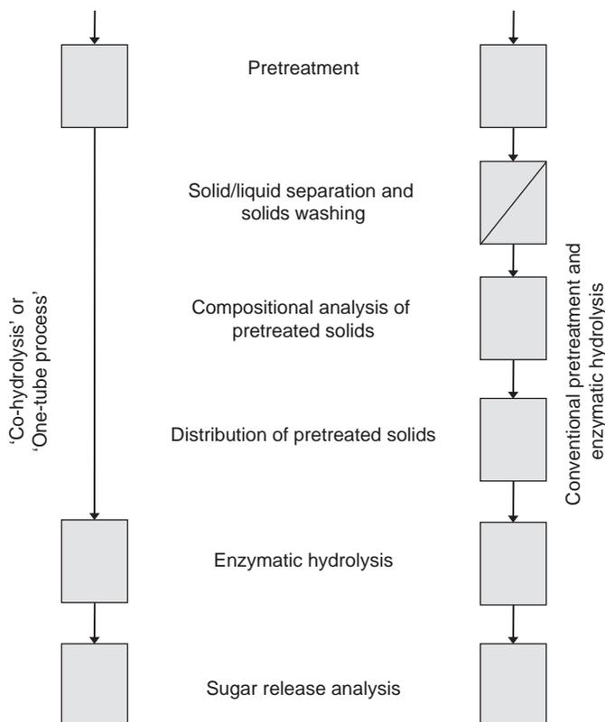
**Figure 22.2** Flow diagrams of conventional pretreatment and enzymatic hydrolysis versus an HTPH approach that employs a co-hydrolysis or one-tube process. (Adapted from Studer et al. [26] © BioMed Central Ltd.).
