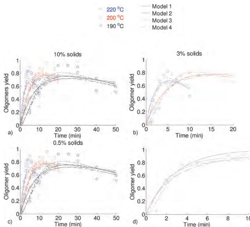
**Figure 4.** Bagasse data parameter fitting: a) batch 10% solids, b) batch 3% solids, c) batch 0.5% solids,<sup>[12b]</sup> and d) FT ( $30 \text{ mL min}^{-1}$ ).
