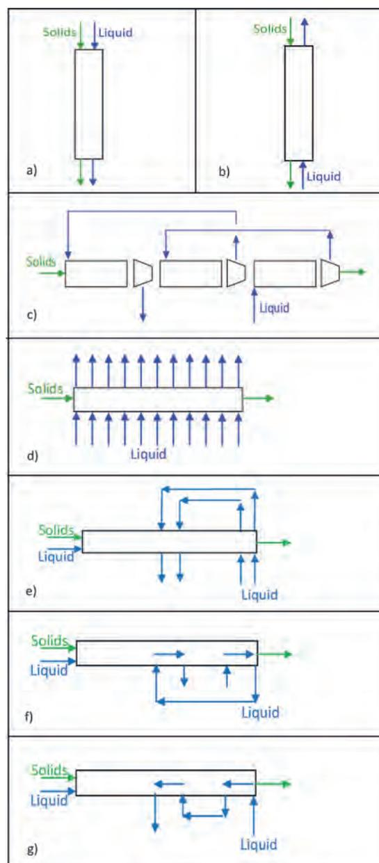
**Figure 5.** Reactor configurations of interest: a) plug flow, b) counter-current (CC), c) discrete counter-current, d) cross flow, e) sequential plug and cross flow (SPC), f) sequential plug and counter-current flow (SPCC), and g) sequential plug and co-current flow (SPCo).
