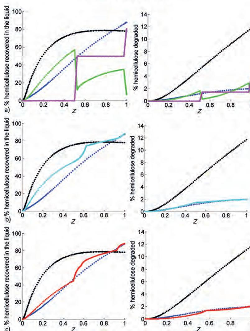
**Figure 7.** Yield of solubilized hemicellulose (left) and degradation products (right) against the fractional progress of the liquid ( $Z$ ) in the reactor using reaction and mass transfer model for plug flow counter-current and a) sequential plug and cross flow (SPC), b) sequential plug and counter-current (SPCC) flow, and c) Sequential plug and co-current (SPCo) flow.
