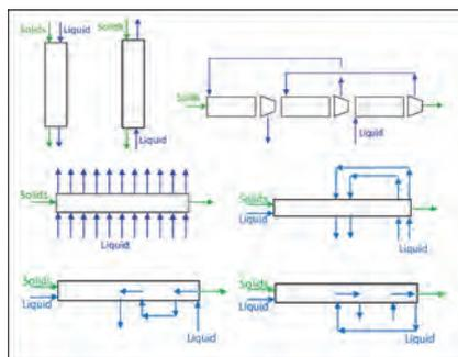
**Bagasse bonus:** The production of fuel from lignocellulosic biomass is of interest to develop a sustainable global energy system. Sugarcane residues such as bagasse are a particularly promising feedstock, but bagasse requires pretreatment. Simulated results show that a variety of promising flow-through pretreatment configurations result in very low sugar degradation and very high fiber digestibility for subsequent microbial or enzymatic processing to biofuel.
