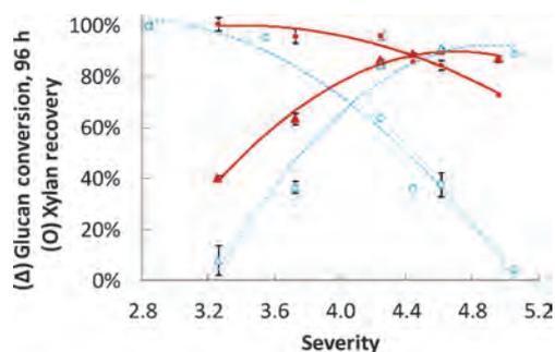
**Figure 1.** Glucan conversion (triangles) and hemicellulose recovery (circles) as a function of severity for different pretreatment configurations for sugarcane bagasse. Open symbols and dotted lines: batch. Closed symbols and solid lines: FT. The error bars show the standard deviation of duplicate measurements.
