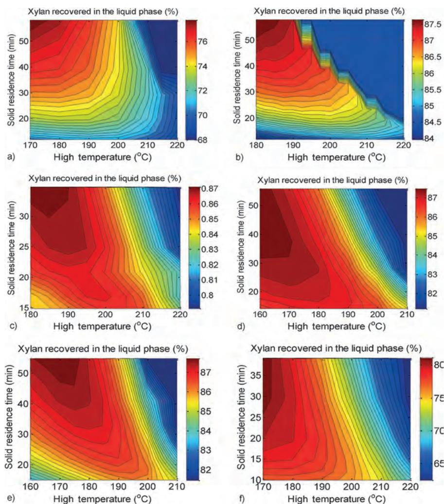
**Figure 6.** Percentage of initial hemicellulose recovered in the liquid phase as a function of solids residence time and temperature if 90% of the hemicellulose is removed from the solids. a) Plug flow, b) CC, c) SPC, d) SPCC, e) SPCo, and f) discrete cc (two stages).
