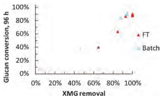
**Figure 2.** Glucan conversion after 96 h of enzymatic hydrolysis against XMG removal after FT- and batch-pretreated bagasse.
