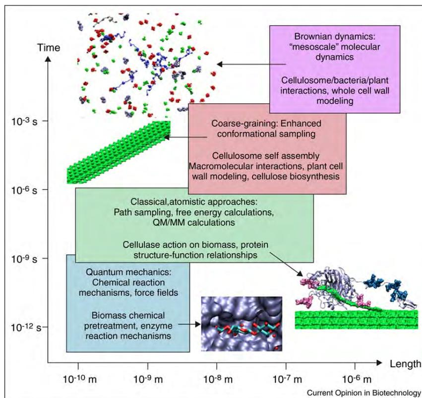
Methods in computational science span multiple spatial and temporal scales from atomic resolution to the application of coarse-graining at multiple resolutions. Listed here are typical techniques applied at various scales with general questions of interest in enzymatic deconstruction of plant cell wall polysaccharides for which computational science can play a role.
