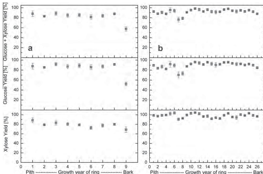
**Fig. 2.** Xylose, glucose, and glucose + xylose yields (%) for the 8 year old (a) and 26 year old (b) cross section. The horizontal axis plots the age of each ring from pith (left) to bark (right), where the final data point represents the bark material. Error bars represent the standard deviation of triplicates.
