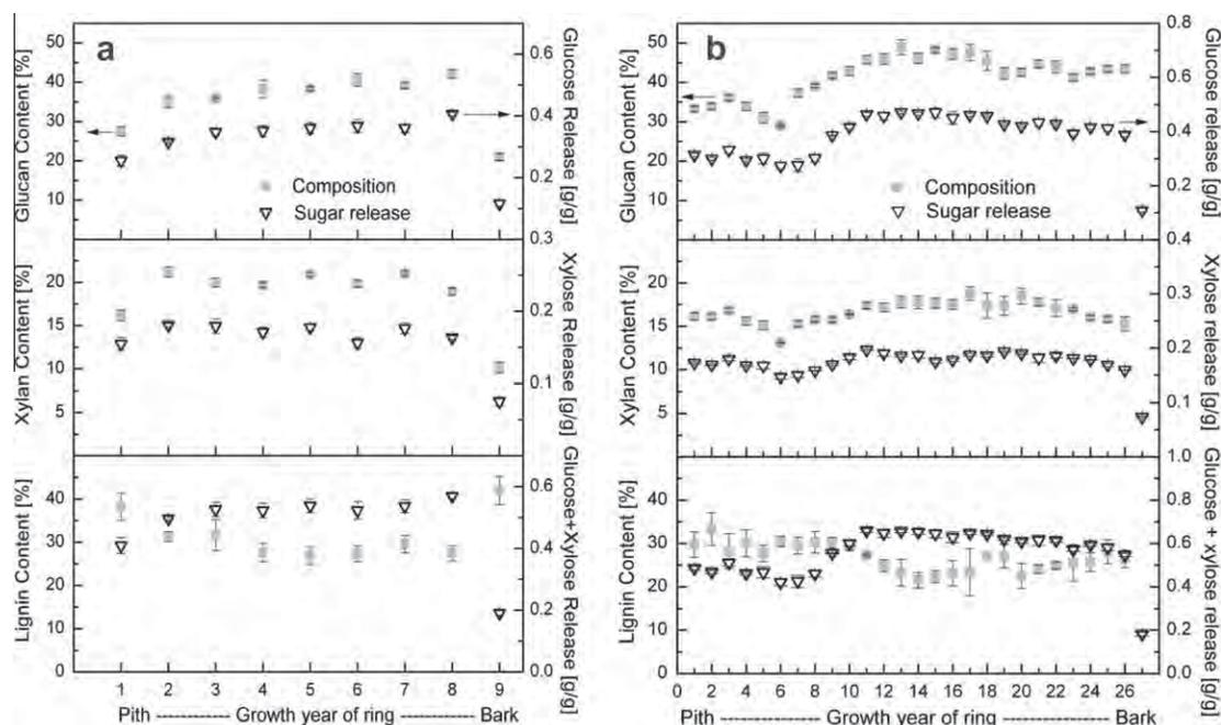
**Fig. 1.** Ring-by-ring composition including glucan, xylan, and lignin contents (in mass percent), as well as ring-by-ring sugar release (in g sugar released/g biomass) for glucose, xylose, and glucose + xylose. Results are shown for the 8 year old (a) and 26 year old (b) section, with the horizontal axis plotting the age of each ring from pith (left) to bark (right), where the final data point represents the bark material. Error bars represent the standard deviation of triplicate experiments.
