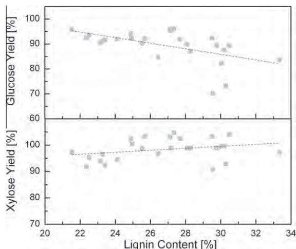
**Fig. 3.** Glucose and xylose yields (%) plotted versus lignin content for the 26 year old section. Dotted lines represent the linear fit of yield data in each subplot to emphasize the observed trends in sugar yields.
