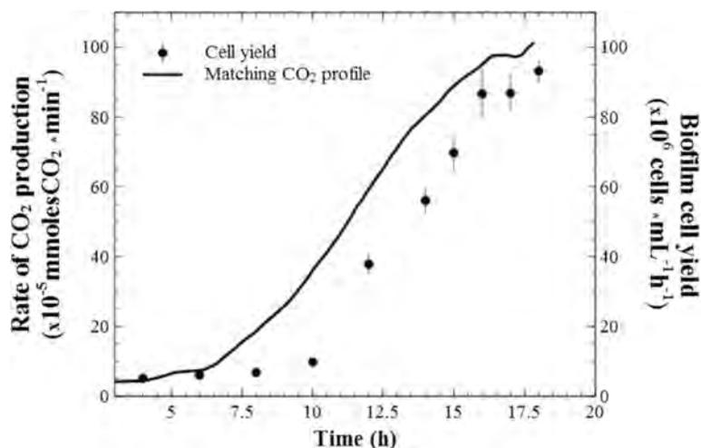
**Figure 7 Biofilm to planktonic cell yield.** Numbers of cells in reactor effluent as indication of biofilm-to-planktonic cell yield and corresponding (matching) CO<sub>2</sub> production rate during the microbial limitation period and a few hours into plateau.
