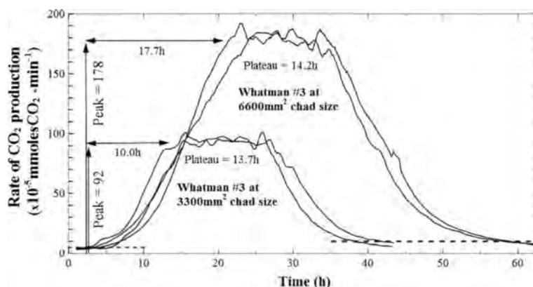
**Figure 9** Rates of CO<sub>2</sub> production during fermentation of Whatman #3 paper chads of 3300 mm<sup>2</sup> and 6600 mm<sup>2</sup> footprint areas. Peak rate doubled, microbial limitation increased and plateau length remained at comparable values for chads with identical thickness but different size.
