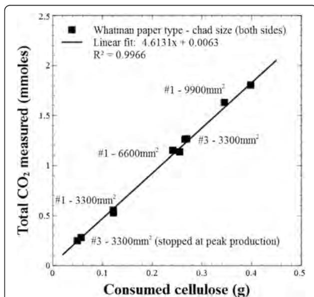
**Figure 2 Correlation between cellulose mass and  $\text{CO}_2$  production.** A strong positive linear correlation was found between the total carbon dioxide measured and the mass of consumed cellulose. Slope  $p = 0.000$ , constant  $p = 0.792$ .
