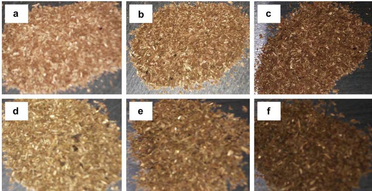
Fig. 2 – Lignocellulosic samples after DAP in a  $\sim 0.10 \text{ mol/m}^3 \text{ H}_2\text{SO}_4$  solution at  $160^\circ\text{C}$  for *Populus* at (a) 2.5, (b) 5, (c) 10 min and switchgrass at (d) 2.5, (e) 5, (f) 10 min.
