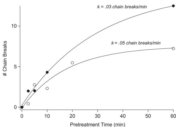
**Fig. 4** – Number of chain breaks per original cellulose chain for (●) *Populus* and (○) switchgrass as a result of DAP in  $\sim 0.10 \text{ mol/m}^3 \text{ H}_2\text{SO}_4$  solution at  $160^\circ\text{C}$ . The lines are fits to an exponential model.
