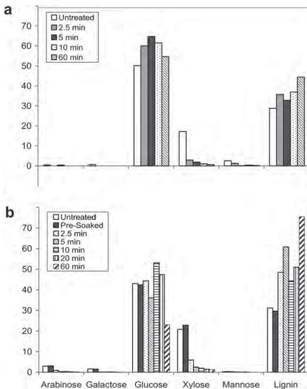
Fig. 3 – Carbohydrate and Klason lignin content of (a) *Populus* and (b) switchgrass after DAP in  $\sim 0.10 \text{ mol/m}^3 \text{ H}_2\text{SO}_4$  solution at  $160^\circ\text{C}$ .
