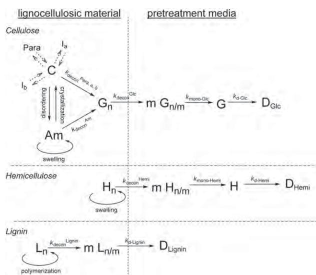
**Fig. 1 – A model that represents the hydrolyzation reactions and probable changes observed in the supramolecular structure of lignocellulosics during DAP (adapted from a figure in Ref. [12]).**
