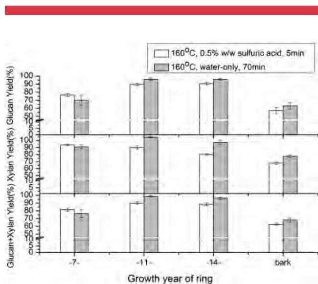
**Figure 4.** Glucan, xylan, and total sugar (glucan + xylan) yields of aspen wood samples 7, 11, 14, and bark pretreated at 160°C with 0.5% (w/w) H<sub>2</sub>SO<sub>4</sub> for 5 min or 160°C with water only for 70 min. The enzyme loading for co-hydrolysis for both was 75 + 25 mg of cellulase + xylanase/g glucan + xylan in raw material. The error bars represent the standard deviation of three replicates for the multi well-plate experiments.
