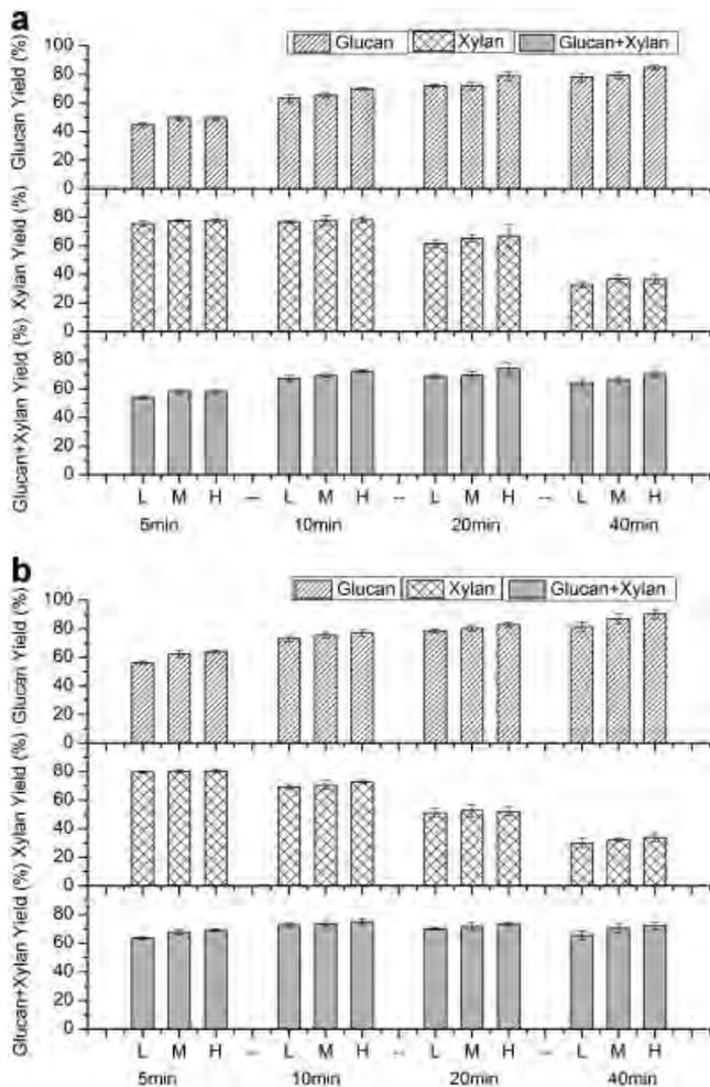
**Figure 3.** Glucan, xylan, and total sugar (glucan + xylan) yields at 5, 10, 20, and 40 min pretreatment times from poplar at 160°C with (a) 0.5% and (b) 1% (w/w) acid concentration. L, M, and H represent enzyme loadings: Low—75 + 25 mg, Medium—105 + 35 mg, and High—145 + 35 mg of cellulase + xylanase/g glucan + xylan in raw material. The error bars represent the standard deviation of three replicates for the multi well-plate experiments.
