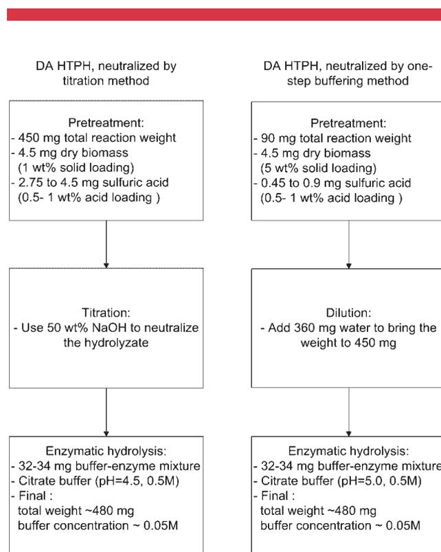
**Figure 1.** Flowchart of thermochemical pretreatment in HTPH system and the neutralization by titration or one-step buffer method.
