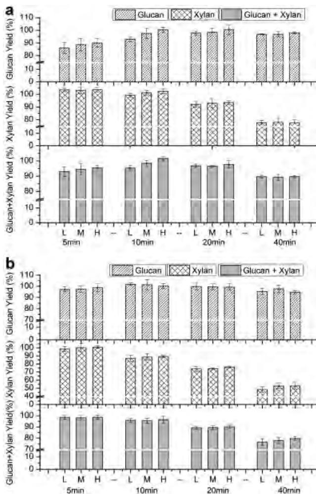
**Figure 2.** Glucan, xylan, and total sugar (glucan + xylan) yields at 5, 10, 20, and 40 min pretreatment from switchgrass at 160°C with (a) 0.5% and (b) 1.0% (w/w) acid loading. L, M, and H represent the following enzyme loadings: Low—75 + 25 mg, Medium—105 + 35 mg, and High—145 + 35 mg of cellulase + xylanase/g glucan + xylan in raw material. The error bars represent the standard deviation of three replicates for the multi well-plate experiments.
