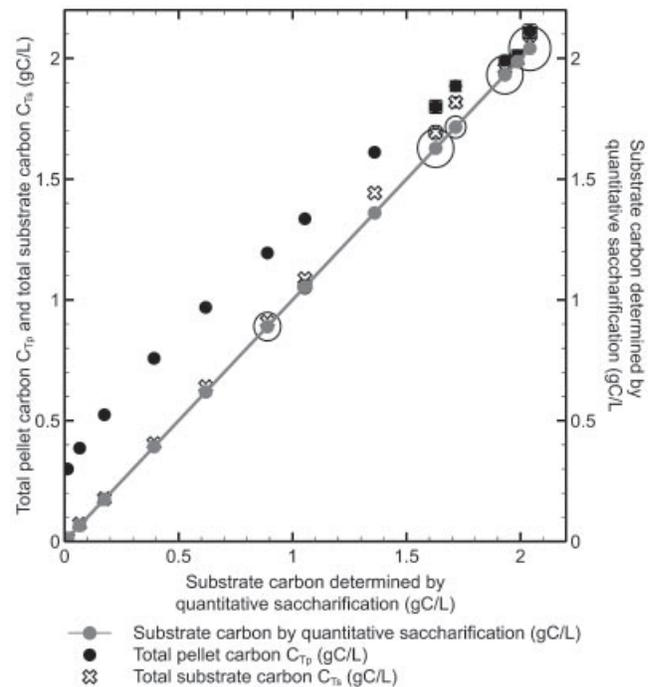
**Figure 4.** Total pellet carbon and total pellet carbon minus biosynthetic carbon compared to residual substrate as determined by quantitative saccharification. The solid grey line with solid grey circles represents quantitative saccharification data, the amount of total pellet carbon ( $C_{Tp}$ ) is shown as black solid circles and substrate carbon ( $C_{Ts} = C_{Tp} - C_{Tb}$ ) is shown as open crosses. The course of the fermentation is from right to left.
