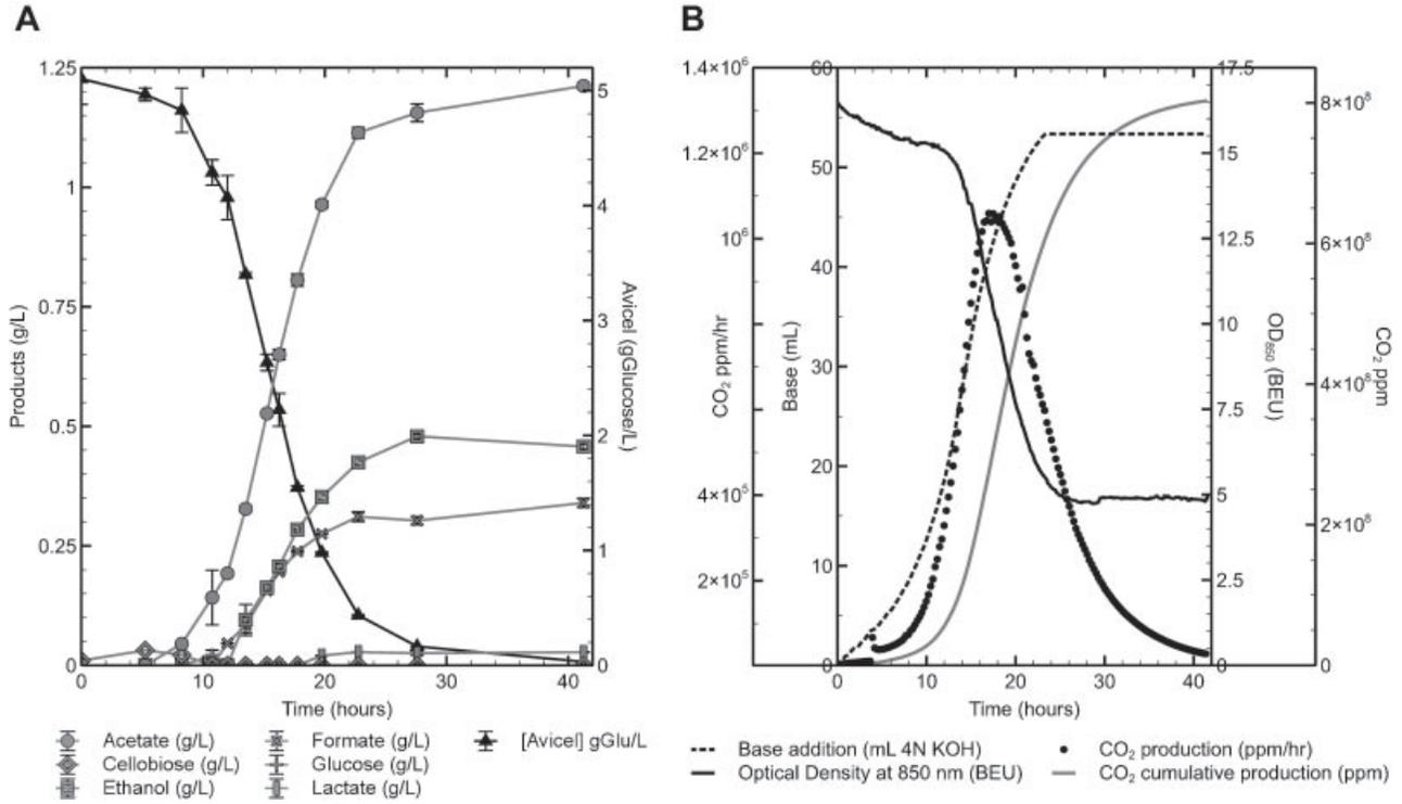
**Figure 2.** Fermentation time course for *C. thermocellum* grown on Avicel (PH105) in LC medium. **A:** Fermentation products and residual substrate concentration. **B:** On-line signals: base addition, CO<sub>2</sub> production rate, cumulative CO<sub>2</sub> production, and OD<sub>850</sub>.
