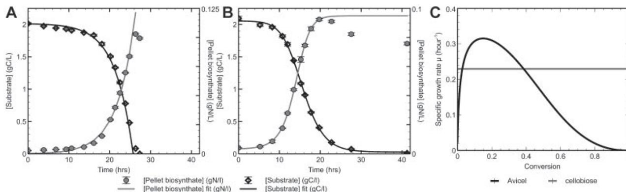
**Figure 5.** Experimental data and fit curves for residual substrate and biosynthate for cellobiose (A) and Avicel (B), and the specific growth rates for both substrates as a function of fractional substrate conversion (C). Biosynthate and residual substrate (Avicel) curves are fitted based on elemental analysis data (see text). Residual cellobiose concentration is determined by HPLC and fitted according to Equation (3).
