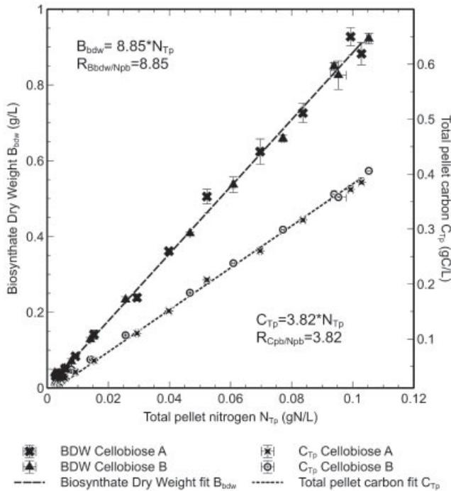
**Figure 3.** Pellet nitrogen versus biosynthetic dry weight (BDW) and total organic carbon in the pellet from two batch fermentations (fermentations A and B) of 5g/L cellobiose by *C. thermocellum*.
