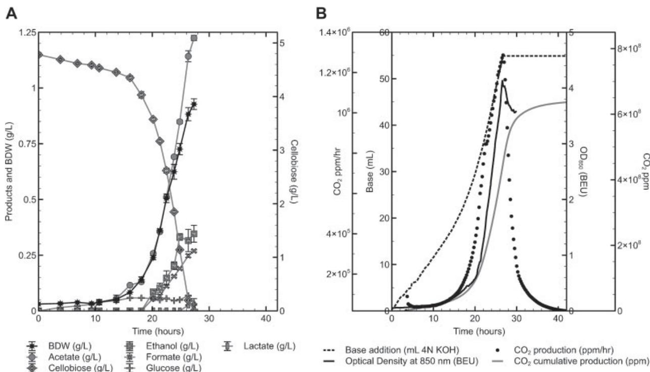
**Figure 1.** Fermentation time course for *C. thermocellum* grown on cellobiose in LC medium. **A:** Biosynthate dry weight (BDW), products, and residual substrate concentration. **B:** On-line signals: base addition, CO<sub>2</sub> production rate, cumulative CO<sub>2</sub> production, and OD<sub>850</sub>.
