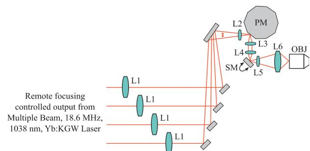
**Figure 2** (online color at: [www.biophotonics-journal.org](http://www.biophotonics-journal.org)) Four beam video-rate imaging system layout. L1: 400 mm Lens, L2: 100 mm Lens, L3: 40 mm Lens, L4: 40 mm Lens, L5: 35 mm Lens, L6: 200 mm Lens, SM: Scan Mirror, PM: Polygonal Mirror, OBJ: Objective.
