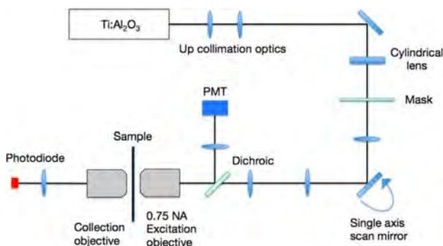
**Figure 10** (online color at: [www.biophotonics-journal.org](http://www.biophotonics-journal.org)) Spatially modulated, line cursor excitation multiphoton microscope schematic. The excitation course is an extended cavity  $\text{Ti:Al}_2\text{O}_3$  oscillator operating at 23 MHz.
