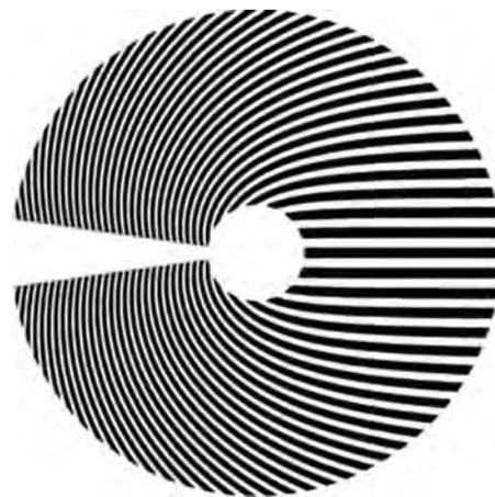
**Figure 11** Mask pattern which is used to create the spatially chirped intensity modulation on the excitation beam.
