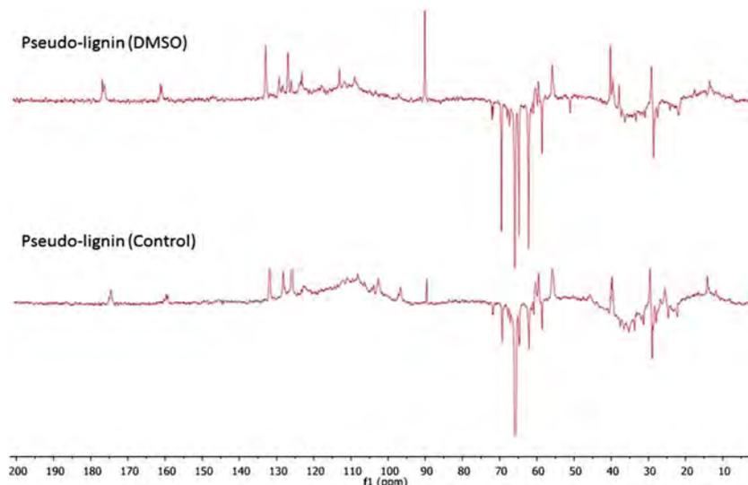
Fig. 4 DEPT-135 NMR spectra of pseudo-lignin (DMSO) and pseudo-lignin (control).
