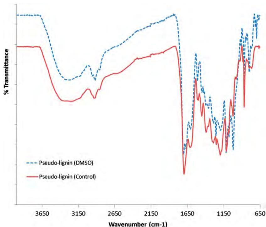
Fig. 2 FT-IR spectra of pseudo-lignin (DMSO) and pseudo-lignin (control).
