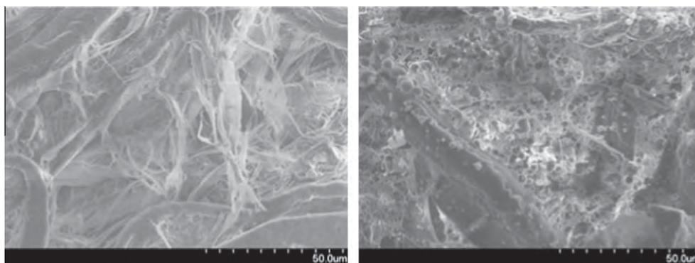
Fig. 1. SEM images of Whatman #4 filter paper samples containing 0% lignin (left) and 30% lignin (right).
