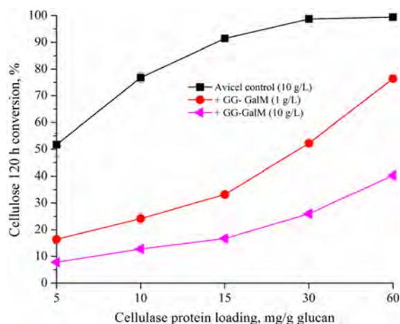
**Figure 4.** Cellulose conversion vs. Accellerase<sup>®</sup> 1500 cellulase protein loadings for Avicel cellulose alone (control; 10 g/L) and Avicel cellulose mixed with guar gum (GG) galactomannan (GalM) at 1.0 and 10 g/L. Note: Enzymatic hydrolysis was performed in a 50 mM sodium citrate buffer (pH 5.0) at 50°C and 150 rpm for 120 h. GG-GalM was added to the hydrolysis slurry before cellulase addition.
