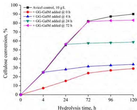
**Figure 8.** Percentage cellulose conversion versus hydrolysis time (h) for Avicel cellulose (10 g/L) alone and Avicel cellulose mixed with guar gum (GG) galactomannan (GalM; 2.5 g/L) added at various hydrolysis time points of 0, 4, 24, and 72 h. Note: Enzymatic hydrolysis in all cases was performed in a 50 mM sodium citrate buffer at 50°C and 150 rpm at an Accellerase<sup>®</sup> 1500 cellulase loading of 15 mg protein/g glucan.
