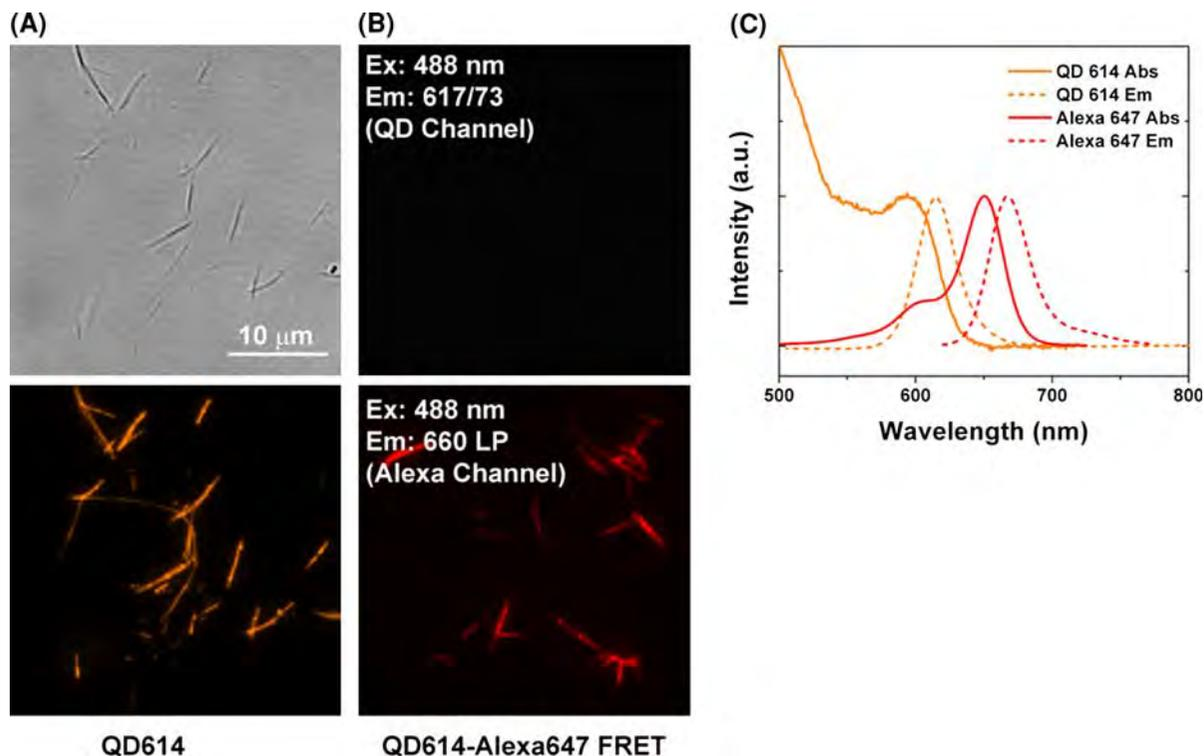
**Fig. 2** Photomicrographic images of fluorescently tagged *CrCBM3* on *Valonia* cellulose. **a** QDs are anchored on *CrCBM3* proteins by the histidine-tags fused at both *N*- and *C*-termini. Bright field image on the *top* showing cellulose, and fluorescence image in the *bottom panel*; **b** images obtained from the microscope channels transmitting only QD (*top*) and Alexa (*bottom*) fluorescence, respectively. The excitation laser wavelength 488 nm can only excite QD but not Alexa. The
