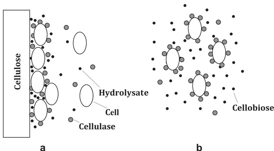
Fig. 1 – Illustrative distributions of cell, cellulase, hydrolysate and cellobiose in a) cellulose- and b) cellobiose-fed cultures.
