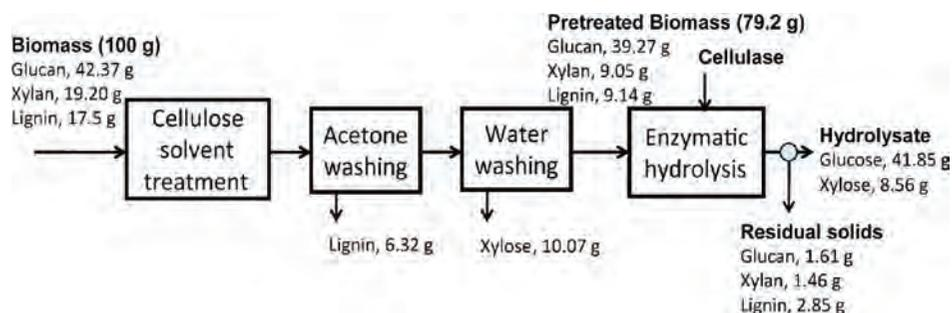
**Figure 5.** Mass balance of industrial hemp hurds after lignocellulose fractionation pretreatment and enzymatic hydrolysis. The pretreatment reaction condition was 84.0%  $\text{H}_3\text{PO}_4$  at 50 °C for 1 h. The enzymatic hydrolysis condition was the same as that in **Figure 1**.
