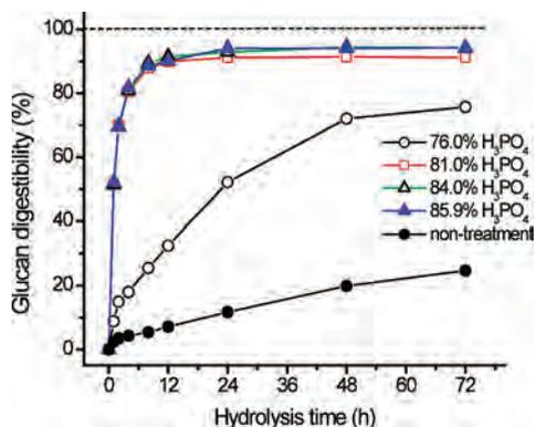
**Figure 1.** Effect of the phosphoric acid concentration on enzymatic glucan digestibility. Pretreatment reaction conditions: different phosphoric acid concentrations at 50 °C for 1 h. Enzymatic hydrolysis condition: 10 g/L glucan, 15 FPU cellulase, and 60 IU  $\beta$ -glucosidase per gram of glucan in 50 mM citrate buffer (pH 4.8) at 50 °C.
