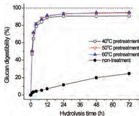
**Figure 3.** Effect of the pretreatment temperature on enzymatic glucan digestibility. Pretreatment reaction conditions: 84.0%  $\text{H}_3\text{PO}_4$  at 40, 50, and 60 °C for 60 min. The enzymatic hydrolysis condition was the same as that in **Figure 1**.
