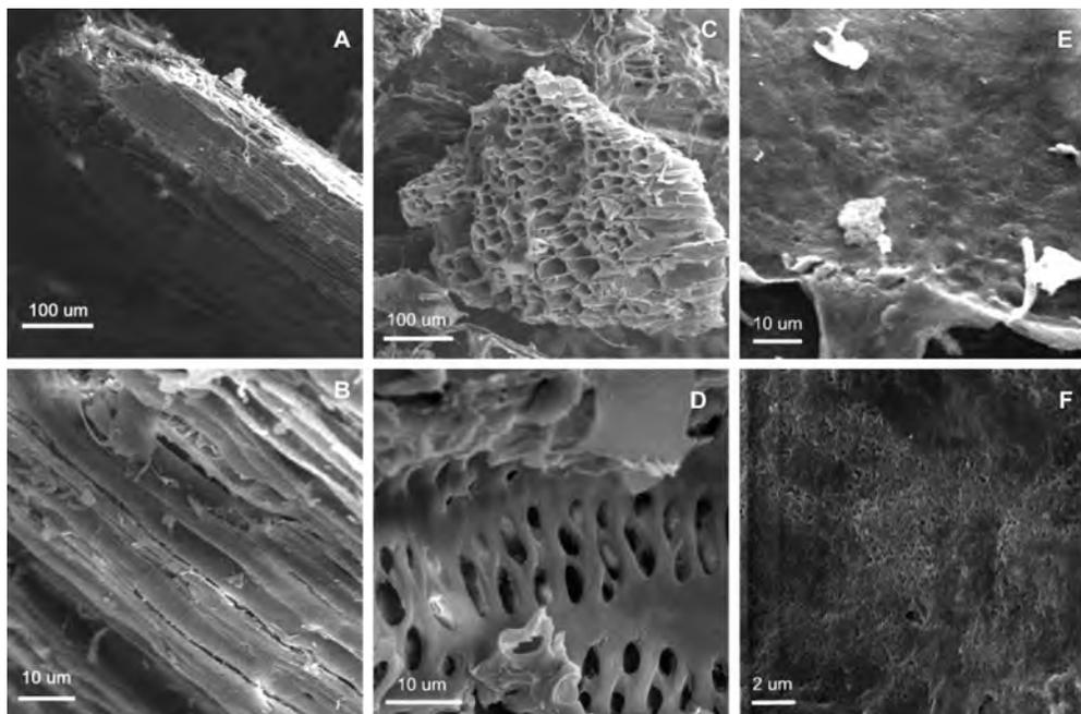
**Figure 4.** Scanning electron microscopic images of industrial hemp hurds at two magnitudes. A and B, the intact sample; C and D, the modestly pretreated sample at 84.0%  $\text{H}_3\text{PO}_4$  at 50 °C for 30 min; and E and F, the well-pretreated sample at 84.0%  $\text{H}_3\text{PO}_4$  at 50 °C for 60 min.
