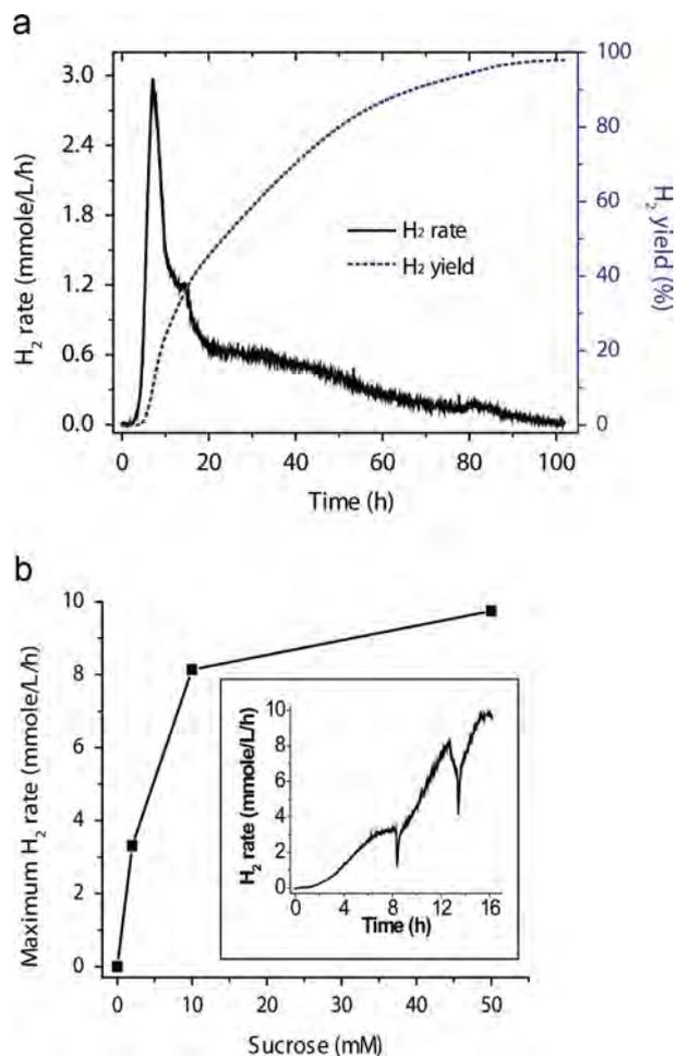
**Fig. 3.** The profile and yield of dihydrogen generation from 2 mM sucrose, 4 mM Pi and 4 mM (Pi)<sub>6</sub> at 37 °C (a) and the maximum hydrogen generate rate in terms of substrate concentration in a fed-batch experiment (b). The reaction buffer was composed of 100 mM HEPES (pH 7.5), 4 mM NADP<sup>+</sup>, 0.5 mM thiamine pyrophosphate, 10 mM MgCl<sub>2</sub> and 0.5 mM MnCl<sub>2</sub>, along with the fifteen enzymes.
