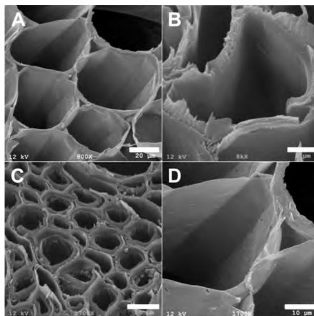
**Figure 3.** Scanning electron microscopy (SEM) images of parenchyma cells of raw switchgrass stem (A and B) and xylem fiber cells of hybrid poplar wood (C and D). The scale bar for panel A is 20 μm; panel B is 2 μm; and panels C and D are 10 μm.
