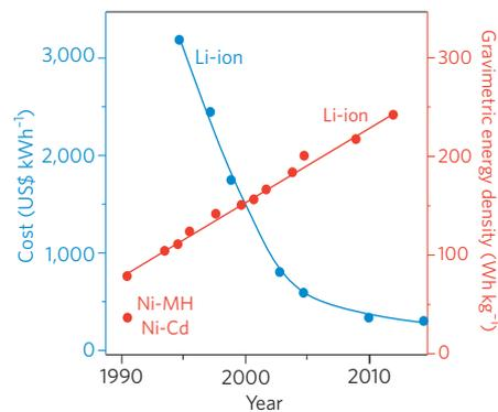
**Figure 3** | Performance and cost of lithium-ion batteries since their commercialization in 1991. The energy densities of rechargeable nickel–metal hydride (Ni–MH) and nickel–cadmium (Ni–Cd) batteries, the best available in 1991, are shown in the lower left corner. Figure adapted from ref. 24, Materials Research Society.
