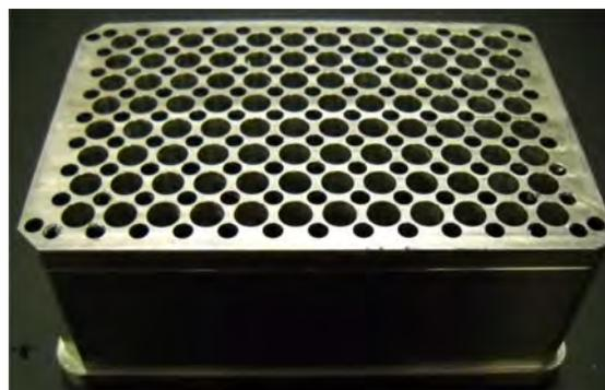
**Fig. 1** Deep well Hastelloy compositional analysis reactor plate with dimensions of 128 × 86 × 51 mm; well diameters are 6.8 mm. The larger openings are the samples wells (96 at 1.8 ml capacity each). The smaller openings are steam channels that are contiguous between the reactor plate clamping system and stacked reactors
