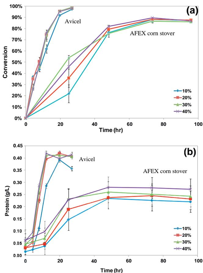
Fig. 3. *C. thermocellum* fermentation using Avicel and AFEX CS with various sizes of inoculation 10%, 20%, 30%, 40% v/v. (a) glucan conversion, (b) pellet protein (cell growth); substrate is 4.4 g/L glucan; AFEX CS was milled to pass a 0.5 mm sieve.
