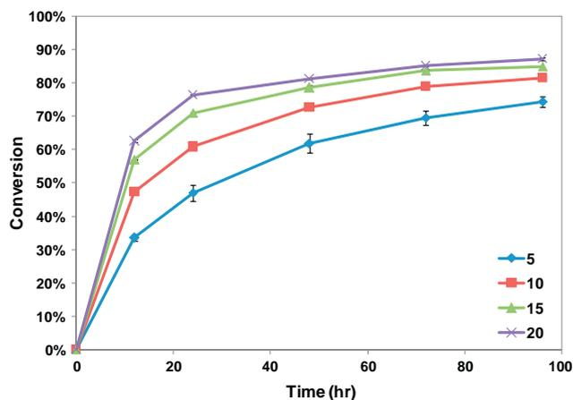
Fig. 2. Glucan conversion for SSF using AFEX CS with various cellulase loadings 5, 10, 15, 20 FPU/g glucan; substrate is 4.4 g/L glucan; AFEX CS was milled to pass a 0.5 mm sieve.
