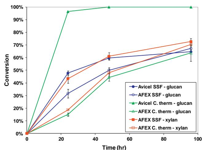
Fig. 1. Conversion for SSF and *Clostridium thermocellum* (*C. therm*) fermentation using AFEX CS and Avicel: substrate is 4.4 g/L glucan; cellulase loading for SSF is 10 FPU/g glucan with an activity ratio of 3 for β-glucosidase over Spezyme CP (IU to FPU); inoculation for *C. thermocellum* is 10% v/v grown on Avicel; AFEX CS has a volume weighted average particle size of 1.4 mm (size range 0–6 mm).
