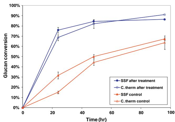
**Fig. 5.** Conversion for SSF and *C. thermocellum* (*C. therm*) fermentation using AFEX CS treated by both hemicellulose removal and particle size reduction (<0.5 mm): substrate is 4.4 g/L glucan; cellulase loading for SSF is 10 FPU/g glucan; inoculation for *C. thermocellum* is 10% v/v grown on Avicel; AFEX CS control has a volume weighted average particle size of 1.4 mm (size range 0–6 mm).
