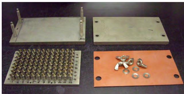
**Figure 1.** Custom-made 96 well-plate with free standing cups attached to a plate is sandwiched between a top and bottom plate together with a flat gasket to seal each well individually. The well-plate has standard dimensions (127.8 mm in length  $\times$  85.5 mm in width) to allow loading with biomass, liquid, and enzymes by robotic tools prior to being clamped together for pretreatment or enzymatic hydrolysis.
