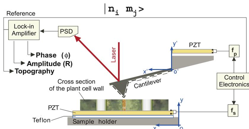
**Figure 1.** Schematic representation of the experimental set-up used for the measurements. The synthesized modes are labeled as  $|n_i m_j\rangle$ , with  $i, j = s, p$  (for sample and probe), and  $n, m = \pm 1, \pm 2, \dots$  corresponding to a given combination of the excitations that yields the mode.
