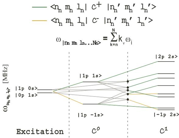
**Figure 2.** Partial diagrammatic representation of the higher level coupling resulting from the tip-sample interaction in MSAFM. The left axis denotes the frequency. The green lines denote modes created via sum frequency generation, while the orange lines correspond to those created via difference frequency generation. The modes arranged in the middle and the last columns are due to first-order and higher-order couplings, respectively. Only mode groups relevant in this work are expanded.
