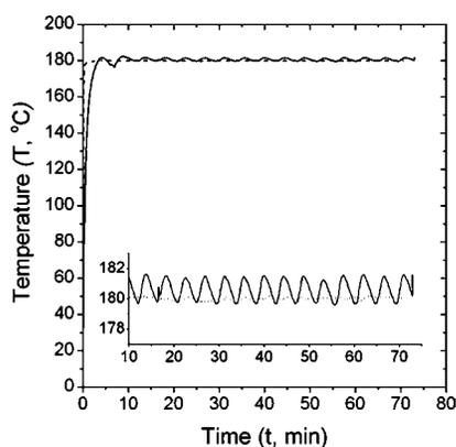
**Figure 1.** Temperature profiles of nine tube reactors during pretreatment at 180 °C for 69.9 min in the fluidized sand bath (solid line) and steam chamber (dotted line). The inset is a magnification of the same data from 10 to 75 s.
