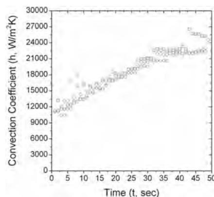
**Figure 4.** Convection coefficient of steam chamber predicted with eq 6 as a function of time. □, run 1; ◇, run 2; ○, run 3.
