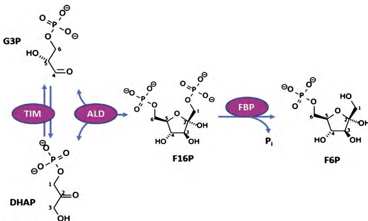
**Fig. 3.** Scheme of the four cascade enzymatic pathway made of triosephosphate isomerase (TIM), aldolase (ALD), and fructose-1,6-bisphosphatase (FBP) containing labile metabolites (e.g., G3P, DHAP, F16P) and stable F6P.
