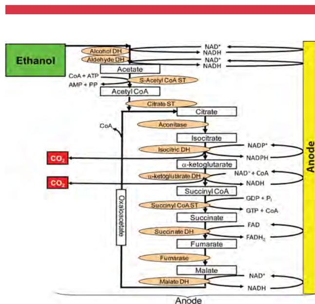
**Figure 5.** The synthetic pathway for complete conversion of ethanol and water to electricity and carbon dioxide (modified by Sokic-Lazic and Minteer, 2008). DH, dehydrogenase; ST, synthetase.
