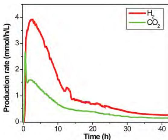
**Figure 4.** Experimental profile for evolution of hydrogen and carbon dioxide from cellopentaose and water.
