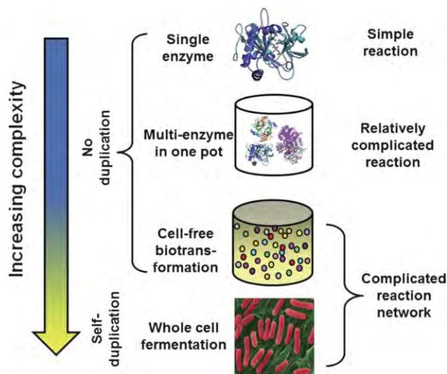
**Fig. 1** Comparison of biocatalysis mediated by a single enzyme, multiple enzymes, cell-free synthetic enzymatic pathway, and whole cells, in an order of increasing complexity.
