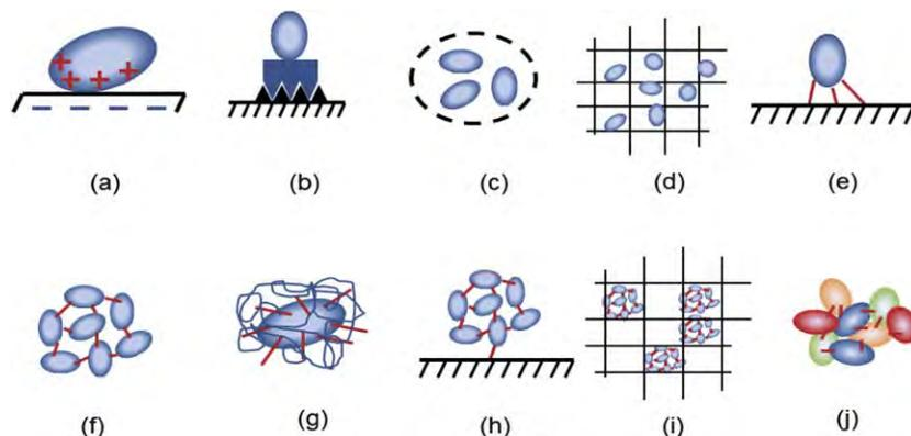
**Fig. 2** General and combined methods of enzyme immobilization: ionic physical adsorption (a), high-affinity physical adsorption (b), encapsulation (c), entrapment (d), covalent binding on an insoluble support (e), cross-linked enzymes (f), a single nano-gel enzyme (g), a combination of e and f (h), a combination of d and f (i), and combi-CLEAs (j).
