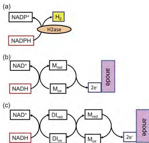
**Fig. 4** NAD(P)H removal by a hydrogenase (a), and electrochemistry through a mediator (b) and a diaphorase and a mediator (c).  $M_{ox}$  or  $M_{red}$ , oxidized or reduced mediator; and DI, diaphorase.
