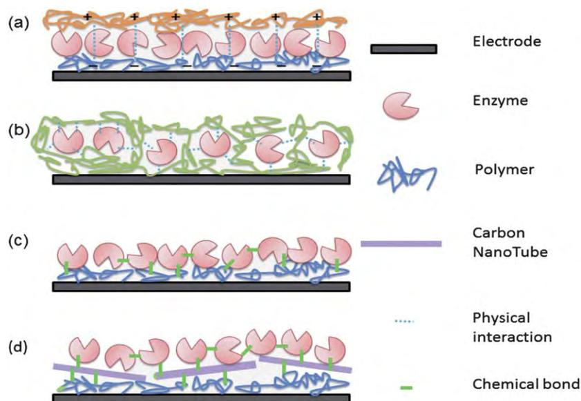
**Fig. 5** Schematic layout of four immobilization methods for redox enzymes on anodes: electrostatic layer-by-layer adsorption (a), entrapment in a matrix (b), chemical cross-linking (c), and chemical cross-linking with CNT (d). The various components are not drawn to scale.
