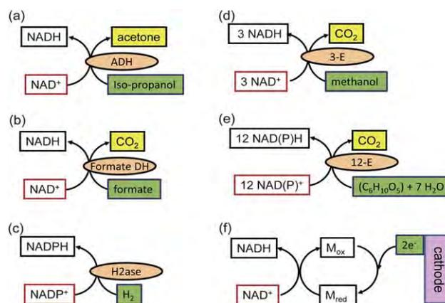
**Fig. 3** NAD(P)H regeneration by a single enzyme (a-c), multiple enzymes containing three enzymes (d), a synthetic pathway containing 12 enzymes (e), and electrochemistry based on an enzyme (f). DH, dehydrogenase; ADH, alcohol dehydrogenase; H2ase, hydrogenase; and  $M_{\text{ox}}$  or  $M_{\text{red}}$ , oxidized or reduced mediator.
